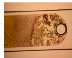
Fig.2 Photograph of latex with calcone. Right side of suspension was irradiated.
