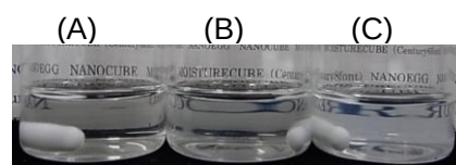
Fig. 1 Sample appearances of cubic liquid crystal based nano-emulsion in C_{12}C_8EO_n /water/glycerin/cetyl ethylhexanoate (CIO): (A) X_s=0.015 , X_o=0.0075 , (B) X_s=0.015 , X_o=0.01 , and (C) X_s=0.015 , X_o=0.015 . X_s and X_o are weight fractions of C_{12}C_8EO_n and CIO in the system, respectively.
