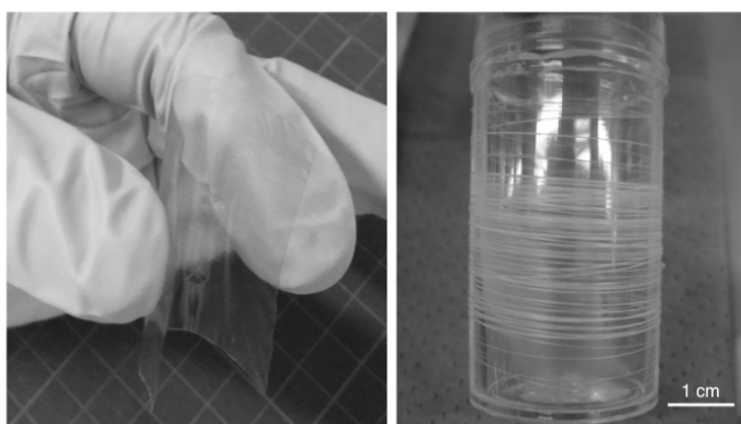
Figure 2. Macroscopic images of the CS/CHI composite film (50 mm square, left) and fiber (right).
